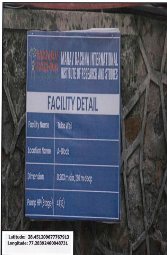
Tubewell Specifications - A Block
