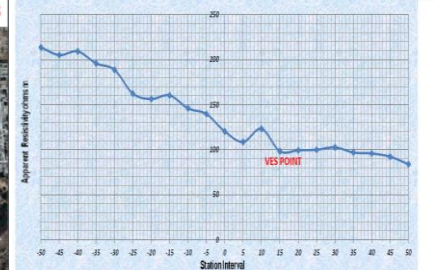
Pseudo Geoelectrical Gradient Profile GRP No-1 N-S direction across Shani Mandir play ground
