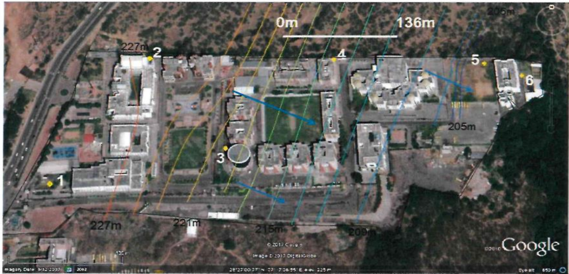
Ground Water Flow Pattern of MRIIRS Campus
