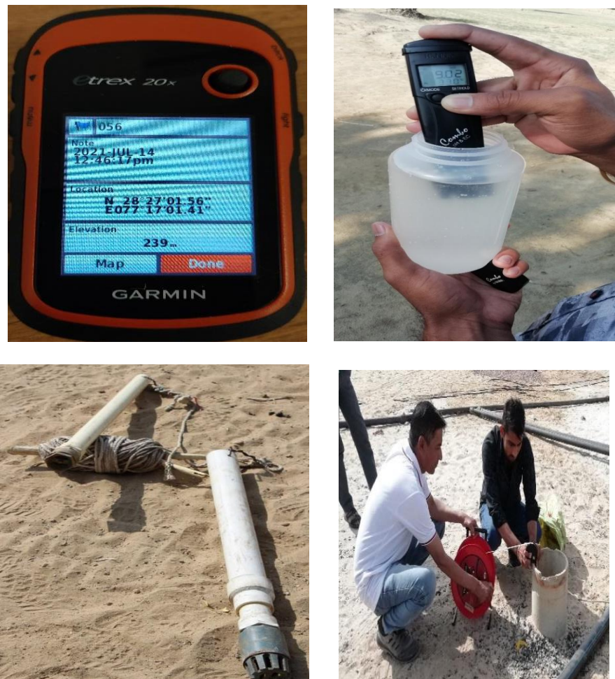
Fig 6.2: Instruments used during field work in Barmer such as GPS, EC- Ph combo meter, water level meter and baller for samples collection.
