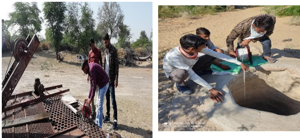
Fig 10.3: Measurement of water level in an open well by water level meter.
